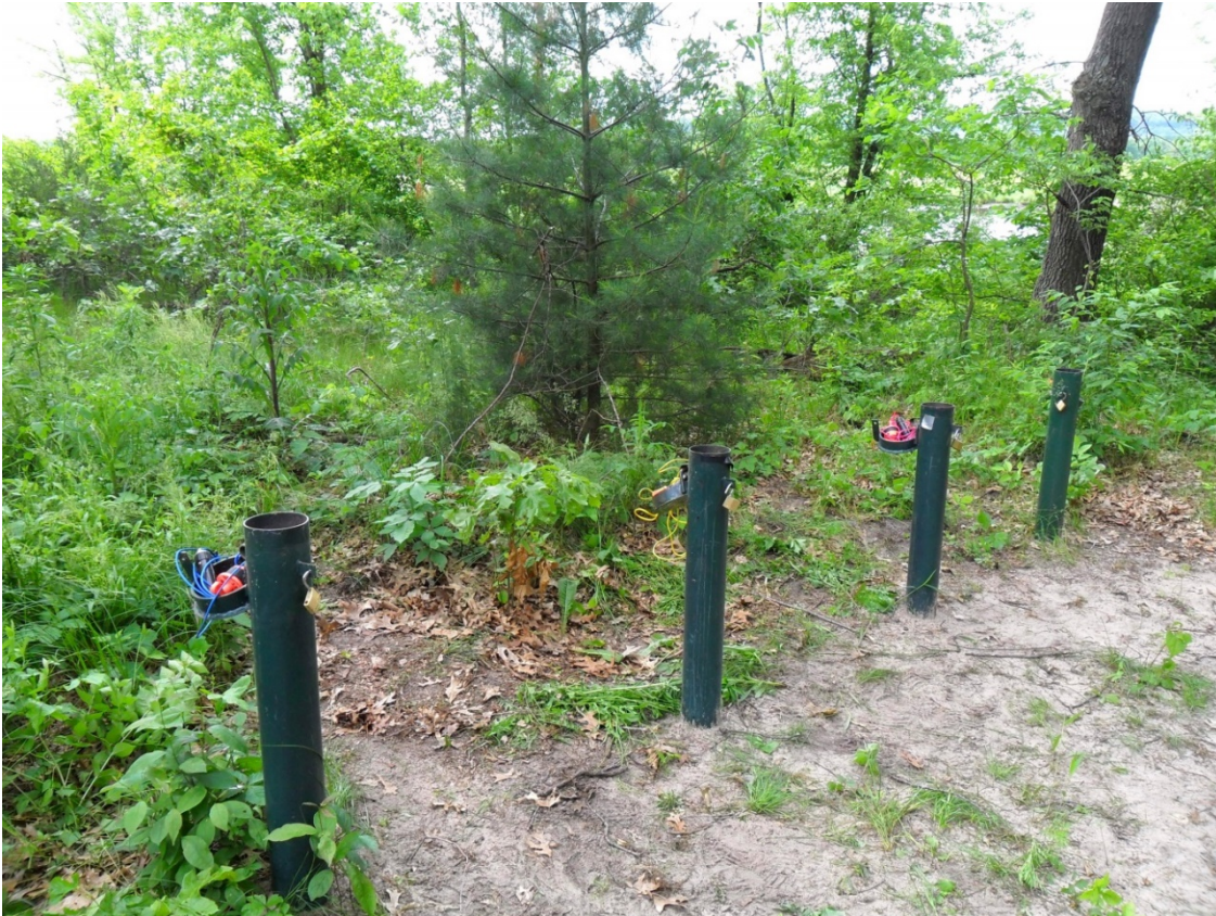
Figure 9. Bakkens Pond well nest showing BP1-BP4. BP5 and BP6 (not pictured) were constructed by the UW-Madison Hydrogeology Field Course.
