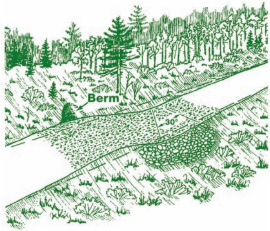
Broad-based Dip Cross-section
