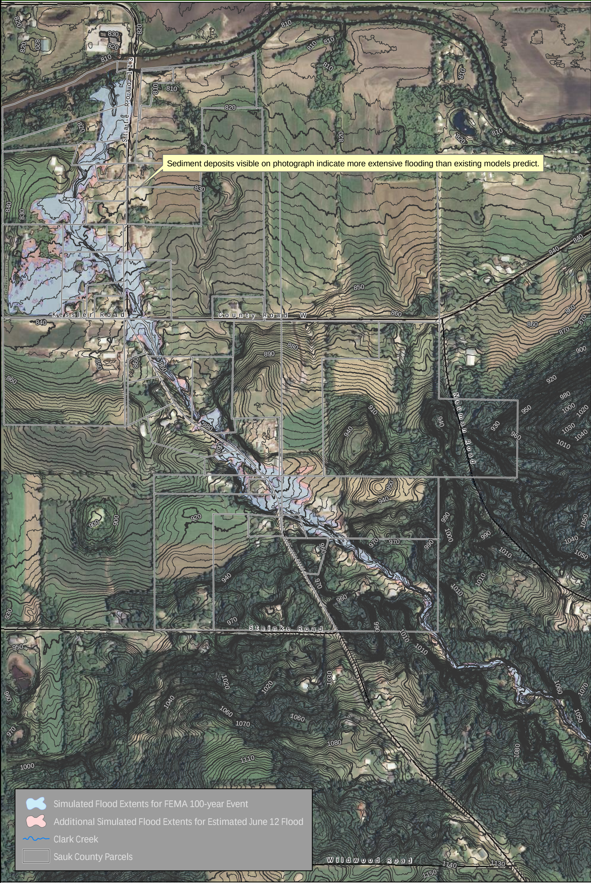
Figure 6: Hydraulic Model Simulation of June 12, 2008 Flood
