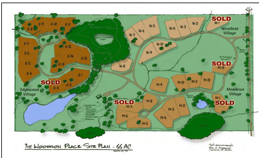
Figure H19 Example of an Actual Conservation Subdivision (Woodson Place, Rains County, Texas)
