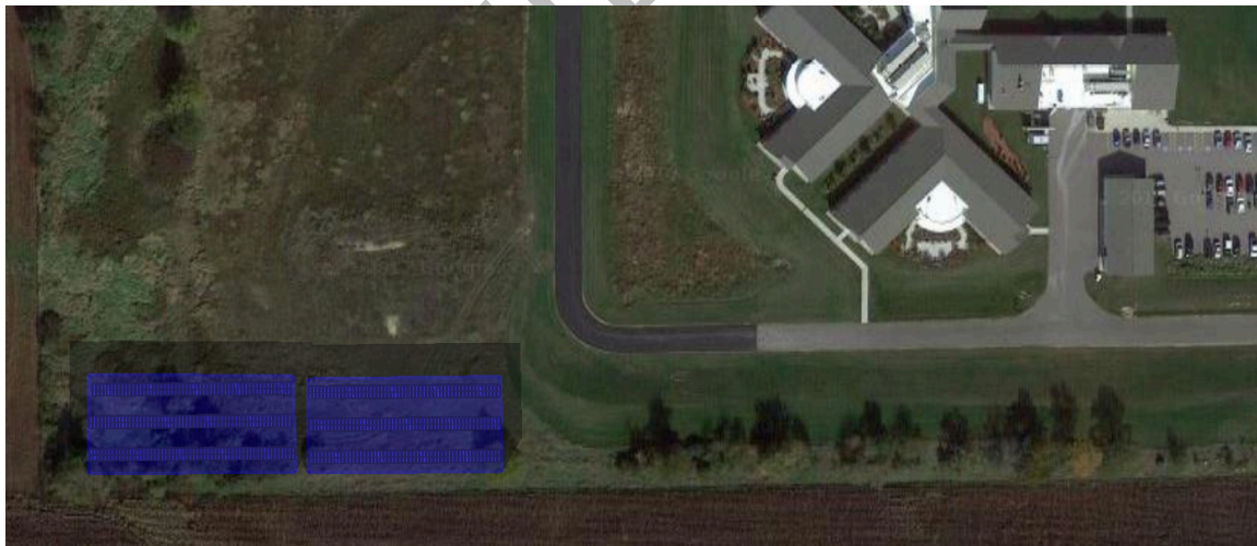
Figure 4. Helioscope Schematic of the Possible Layout for the HCC ~225 kW Solar Arrays
